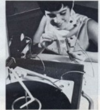
Photograph uses an amplifier (in mode's hand) printed on kitchen foil. In addition to making cheap electronic devices, paper circuits may be printed in books, on credit cards and documents.
